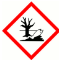
Hazardous to environment
